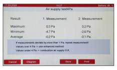
Two measurements (each 4 minutes) will be carried out and the result displayed. A tip is issued for the measurement result. Under "Graphics" a graphical history can be displayed.
