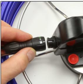
To connect, match the arrow of the bayonet jack with the bayonet plug. Now mount the Camera-Head onto the end of the GRP-Rod and secure with the union nut.
