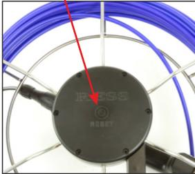
The reel has a digital Meter-Counter which is displayed in the display. The Counter can be reset manually at any time, during the inspection, by touching the reset-field. This is useful if you want to perform a relative measurement. This is possible in both directions.
